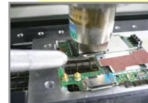
< Removing an IC from the substrate >
